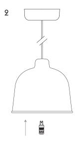
GRAIN PENDANT LAMP G9 SBLED TYPE T, MAX 5W. LED ONLY. 12OV ~ 6OHZ
